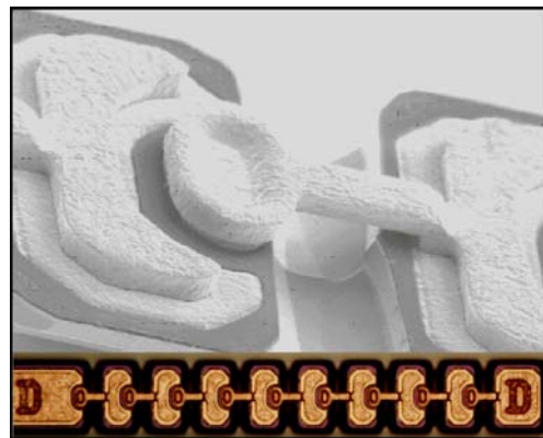
Fig. 2: Photograph and scanning electron micrograph of the D190HP Schottky barrier varactor chips.
